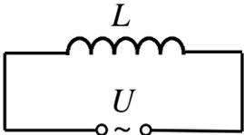
$$I = \frac{U_m}{\omega L} \sin \omega t = I_m \cos \left( \omega t - \frac{\pi}{2} \right),$$
